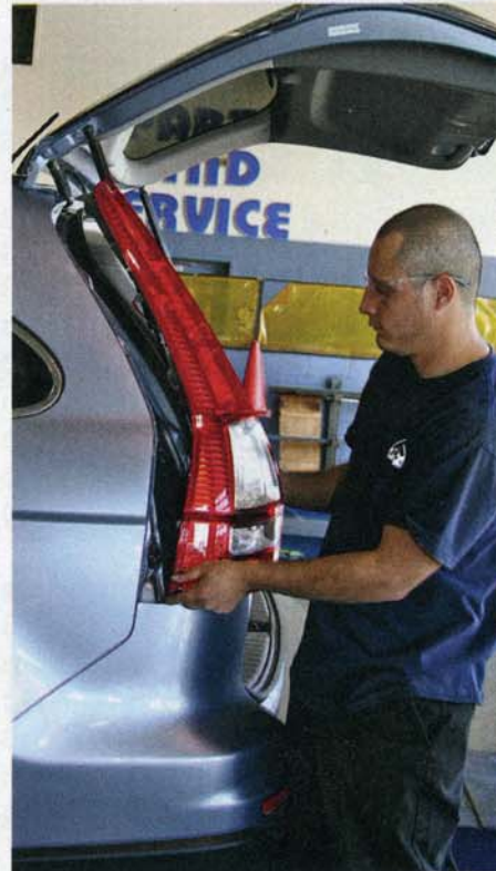
A taillight lens for the CR-V is easily removed, exposing wiring into which diodes are spliced and connected to the motorhome wiring harness.
