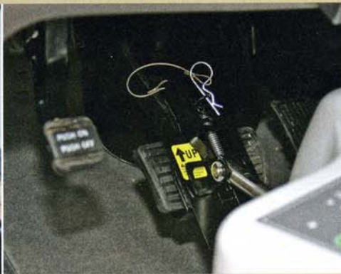
A clamp fitted to the pedal allows the Even Brake to actuate brakes during towing.
