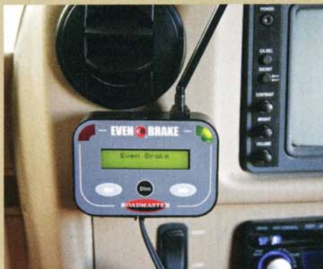
The monitor reflects the status of the Even Brake and signals when brakes are applied.
