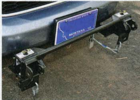
Quick-disconnect assembly adds rigidity for towing and offers easy disassembly, leaving two small receiver tubes visible on the car.
