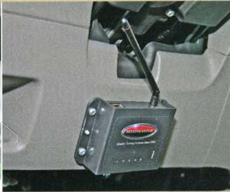
The transmitter relays performance and troubleshooting data to the monitor.
