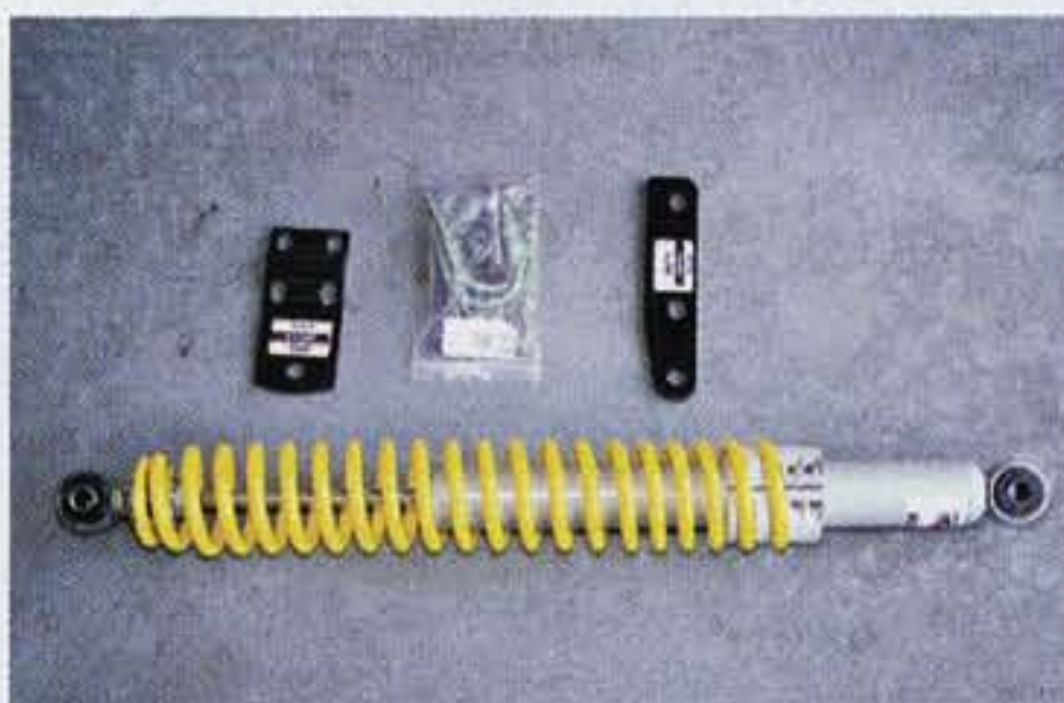
Reflex Steering Stabilizer consists of a steering damper inside a coil spring, designed to return wheels to center.
