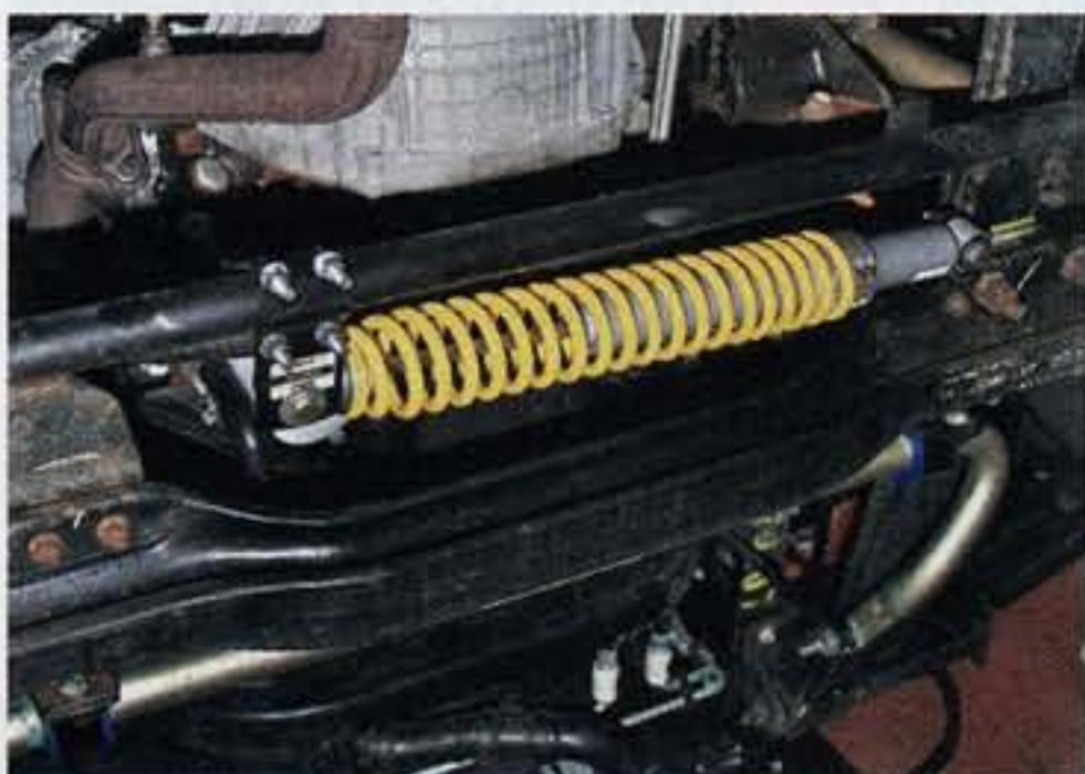
Reflex Steering Stabilizer, bolted to frame (right) behind axle and to steering tie rod (center), exerts spring pressure to re-center steering and dampen steering motion.
