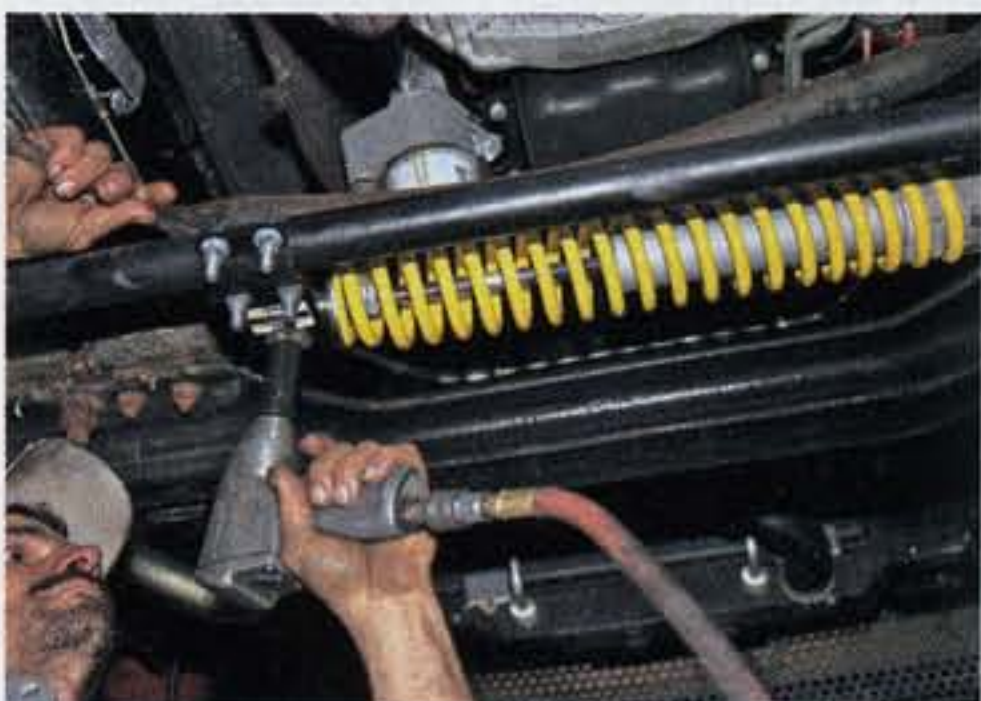
Position of tie rod bracket determines neutral position of stabilizer.
