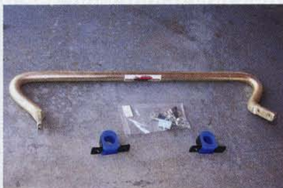
Roadmaster front stabilizer bar replaces stock Ford bar, utilizing polyurethane bushings.
