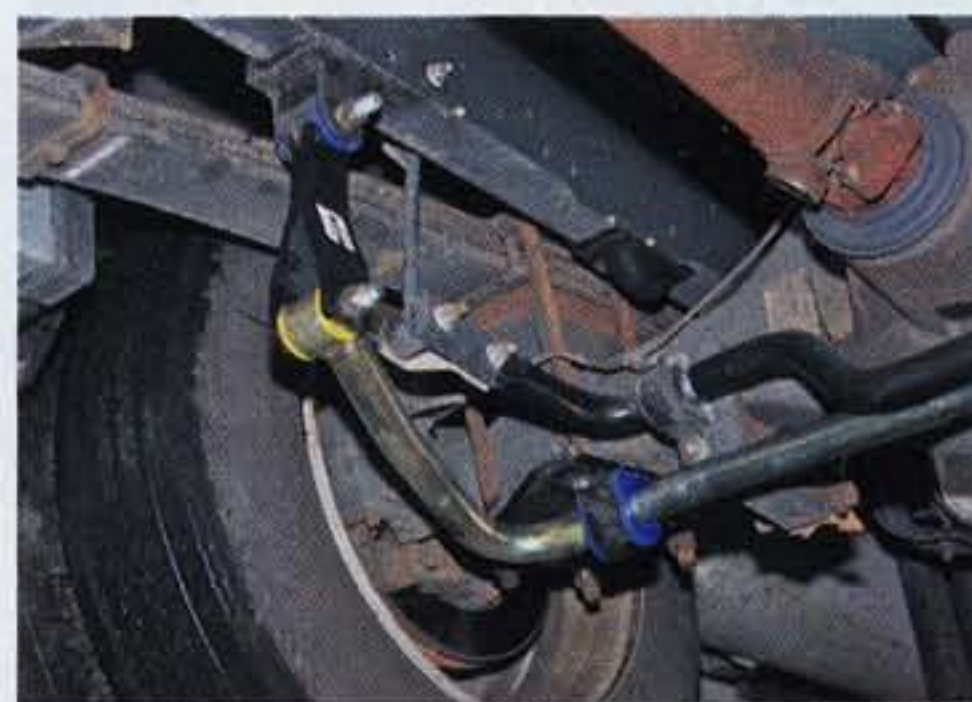
The Roadmaster and Ford rear stabilizer bars are attached to the axle and frame independently, using separate linkage.
