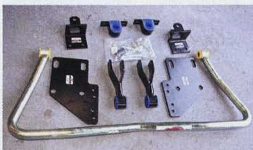
Steel brackets provide a platform left and right for attachment of the Roadmaster bar below the rear axle. U-shaped brackets, center, are bolted to the frame for connection with tips of bar.
