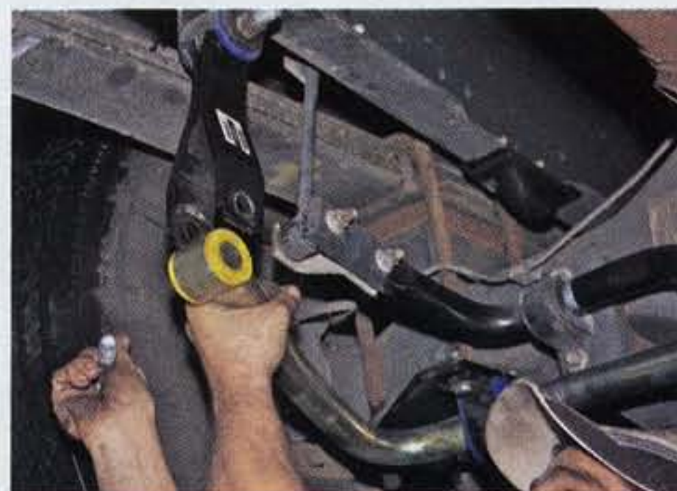
Polyurethane bushings permit less flex between bar and frame brackets.
