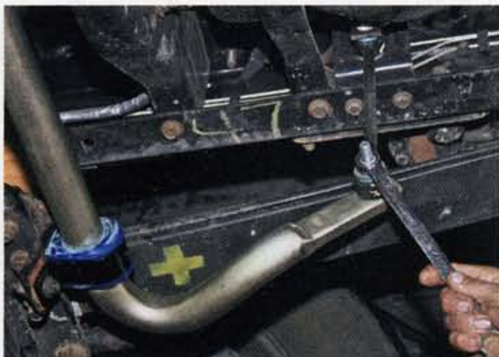
Roadmaster front bar is thicker than stock bar and utilizes stock frame linkage.
