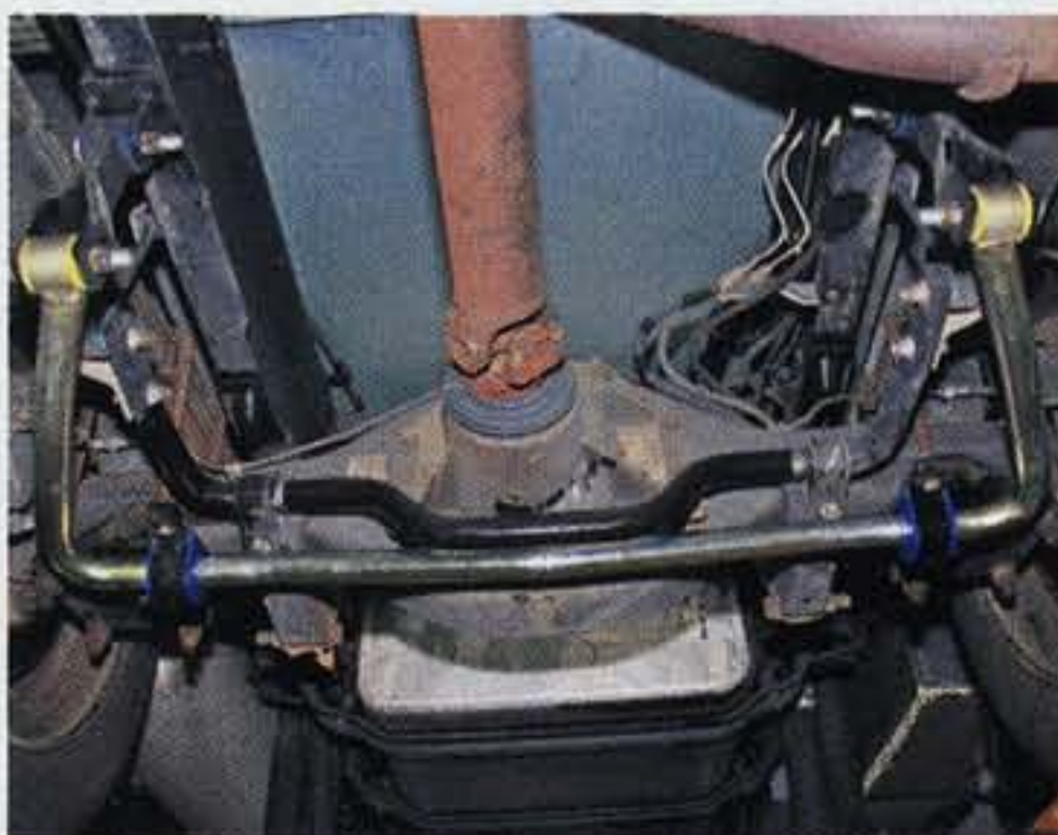
The larger Roadmaster rear bar encircles the stock Ford bar and more than doubles roll resistance.
