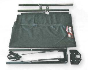
The Tow Defender is a large (72-by-50-inch) panel of vinyl-coated mesh that is secured by steel tubing fore and aft, providing a horizontal barrier between the motorhome and dinghy. Rocks and sand that get by the motorhome's mud flap are deflected down to the road surface.
