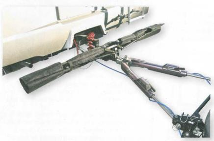
Material rolls up and is strapped in place on the tow bar shank; no need to remove between uses since it doesn't interfere with the tow bar in stored position.
