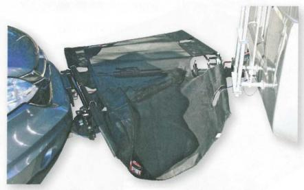
Tubes and struts fold the material for clearance when turning in either direction. Material pops back into place when turn is completed.
